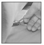
2. Pull up on the strap loop located at the rear of the seat cushion and flip the seat cushion forward.
